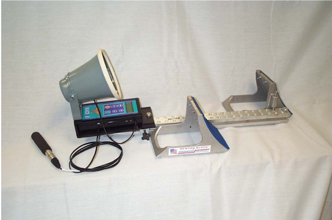
Figure 23: Connected Signal Input and Loudspeaker Cables
