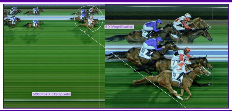
The Vision PRO X extended vertical resolution ensures precise adjudication, even when competitors occupy minimal sensor space, making it ideal for wide racecourses such as in rowing or horse racing.
