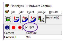
NOTE: The wireless network of the camera is only available when the EVF box is checked
