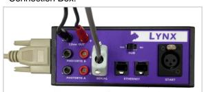
e. When the Gauge is receiving power, the red light next to the XLR port on the Gauge will start to blink.
