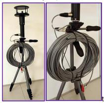
d. Connect the Wind Gauge Input Cable to the serial port and the power leads to the color-coded red and black 12VDC ports on the Vision-Series camera back panel.
