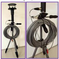
d. Connect the Wind Gauge Input Cable to the Connection Box serial port and the power leads to the color-coded red and black 12VDC ports on the Connection Box.
