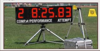
**SeriaLynx** enables fast and secure wireless communication between the FieldLynx computers and the LED display/wind gauge. One unit connects to the LED display to show live marks and standings from FieldLynx while the other connects to the wind gauge to wirelessly pull live wind readings for jumping events.
