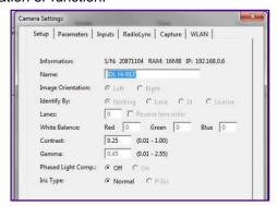
c. Click the **Parameters** tab and set the Frame Rate/Height and shutter speed to your preference.
