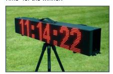
The 9-digit Alphanumeric LED display connects to your FinishLynx system and can display running times and results that are clearly visible from over 200 feet away. The display also integrates with the ACM plugin to automatically display finish times or splits whenever an athlete crosses the finish line.
