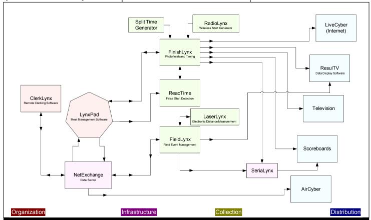
With the addition of **LynxPad** to the Lynx family of products, the data movement process is complete. The above diagram shows how all the components interact by simply sharing files over a computer network. As always, the concept is modular: adding any piece will give more power and versatility to your existing set up.
