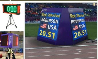
live running times and race results. The 2-sided display also connects directly to the Vision or Vision PRO camera to show live race data and FinishLynx images using the Video Display Module.
