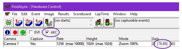
**TIP:** The exposure time (ms) appears between square brackets [] in the **Gain** field of the Hardware Control window.
