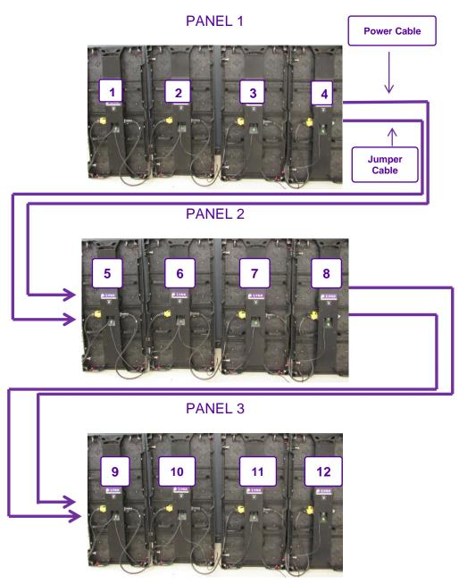
The image above shows the back of the display with the panels wired correctly. Panel 1 has the Power Input and Signal Input. Panel 2 has Power input and Signal Input connected via Panels 4 & 5. Panel 3 has Power Input and Signal Input connected via Panels 8 & 9.
