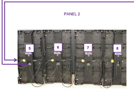
The image above shows the back of the display with the panels wired correctly. Panel 1 has the Power Input and Signal Input. Panel 2 has Power input and Signal Input connected via Panels 4 & 5.
