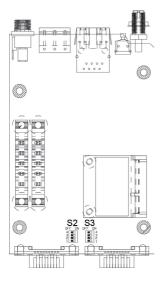
You may need to set the pull-high/low resistors when termination resistors are used in certain RS-422 or RS-485 environments.
