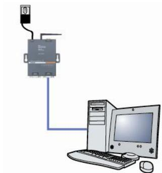
1. Connect one end of the supplied DB9F – DB9F null modem serial cable to the WiBox's serial port 1.
