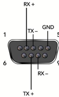
Figure 2-7. RS-485 2-Wire Pinouts
