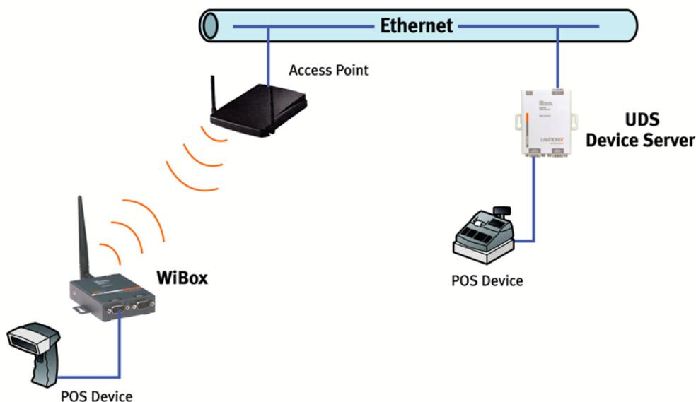
In the example above, the WiBox communicates with another device server via the AP. The UDS device server, in this example, is connected via an Ethernet connection to the AP. In this way, the WiBox and the device server communicate directly and can transfer information between their serial devices.
