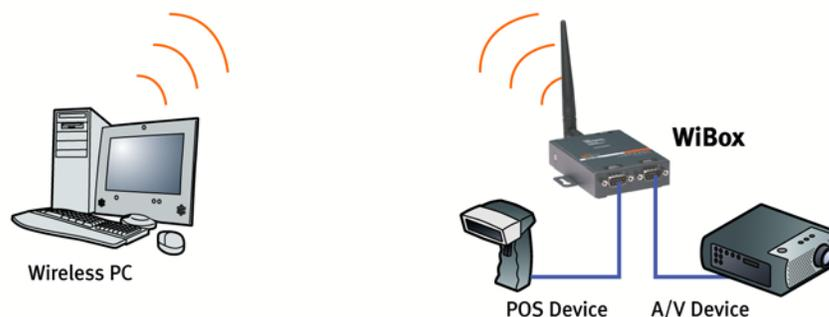
In the example above, the AP is not present. The PC makes a direct wireless connection with the WiBox to manage serial devices. Without an AP, it is a peer-to-peer relationship.
