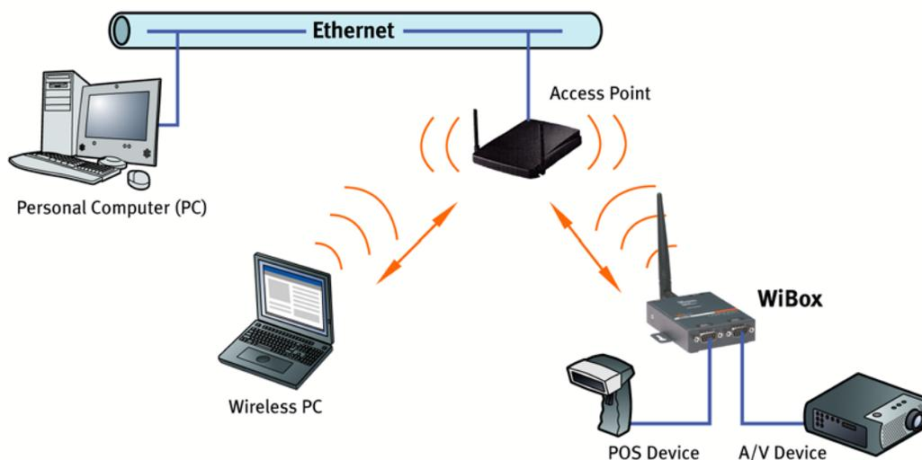
A PC connected to an AP via an Ethernet connection and a PC with a wireless connection to the AP LAN access the WiBox as though they are connected to it directly. The combination of the WiBox, a PC, and Lantronix's Redirector software allows the PC to communicate directly to the WiBox's serial devices, providing wireless serial tunneling.
