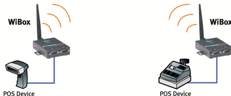
In the example above, two WiBoxes have established an Ad Hoc peer-to-peer relationship. They communicate directly to each other's serial devices without a PC or an AP.
