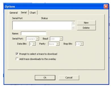
**2** Click the **New** button. A Serial Port is added to the text box, with the status "Not Running."
