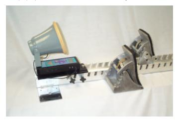
Figure 2: Properly mounted ReacTime unit
