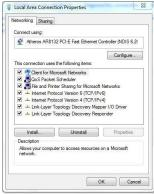
7.) A Properties window will appear and is typically set to Obtain an IP address automatically. Click to select the radio button for **Use the following IP address**. In the box for IP address, enter **192.168.0.5** for FinishLynx and hit Tab key to auto fill in Subnet mask **255.255.255.0** (Meet Management computer will be **192.168.0.90**).
